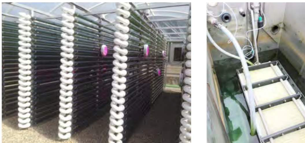
Figure 5-13: Clearas ABNR Pilot (11 gpm) (L: Photobioreactor with LED Lights; R: Flat Sheet Membrane Tank)
