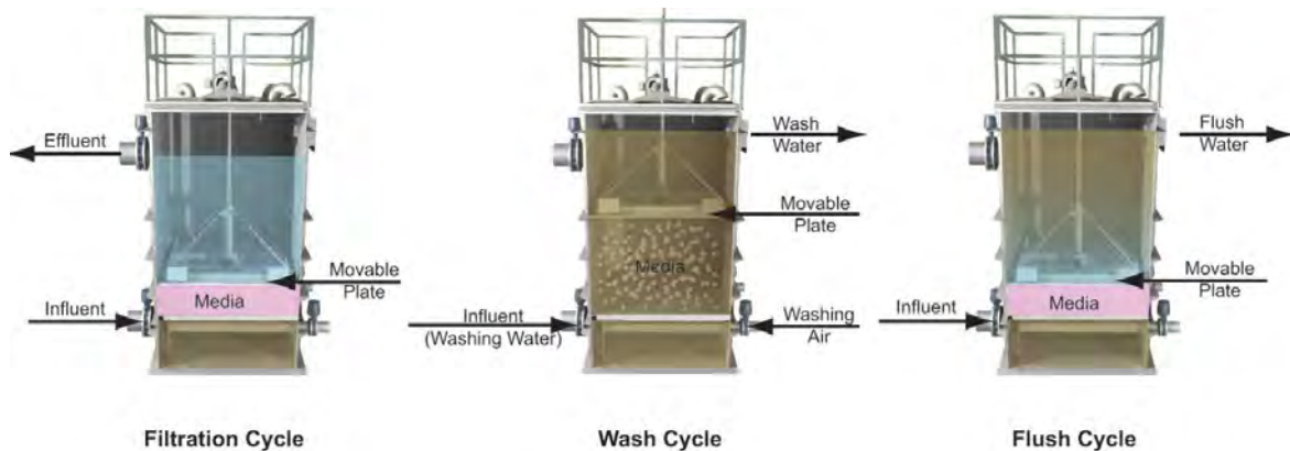
Figure 5-4: Schematic of Schreiber Fuzzy Filter
